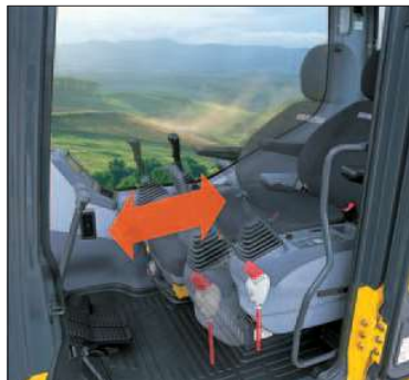
Seat Sliding Amount: 340 mm 13.4", increased 120 mm 4.7"
