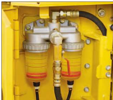
Fuel pre-filter (with water separator) Fuel main-filter Additional fuel main-filter
