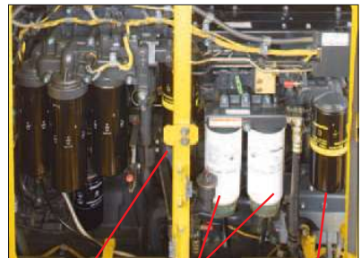
Fuel pre-filter (with water separator) Fuel main-filter Additional fuel main-filter
