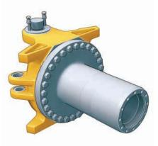
**Articulating/Oscillating Hitch.** The articulating hitch provides the truck with steering articulation, and the oscillation ensures all-wheel ground contact in rough terrain.
