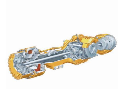
**Inter-Axle Differential Lock.** Locks all three axles in unison and modifies distribution for excellent traction in poor underfoot conditions and on grades. It is operated by a switch located at the footrest. **Cross-Axle Differential Locks.** Provides full driveline locking — all three axles and all six wheels — for maximum performance in the most adverse conditions. Acts in unison with the inter-axle differential lock when the footswitch is actuated and the dashmounted switch is selected.
