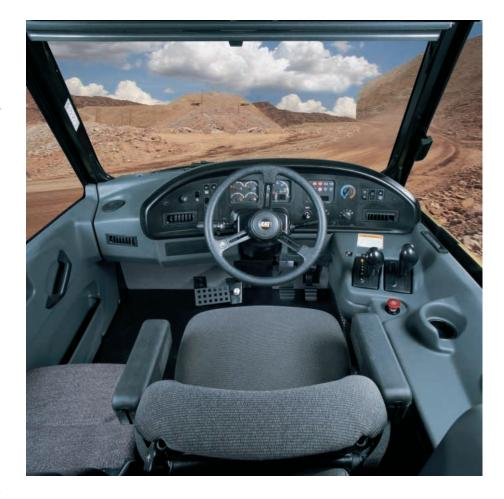
**Suspended Pedals.** The suspended pedals are easier to operate and reach, while creating more leg and foot room. They also make for easier cleaning of the cab floor by keeping the pedals out of the dirt.
